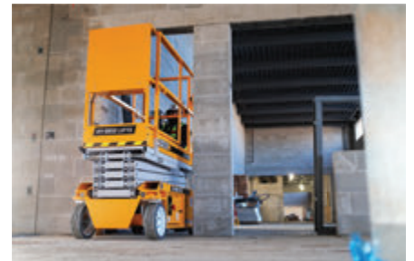
The compact dimensions of the PS-1930 allow the unit to fit through standard doors and elevators without an operator exiting the lift to fold down the rails.
