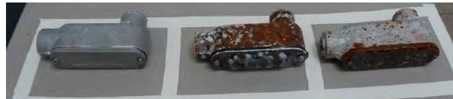
Before and after photographs. Above photo are new conduit bodies and below photo shows same conduit bodies after 42 days in salt fog.
