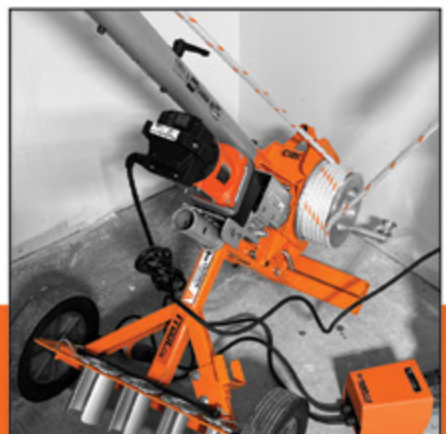
Dual capstans with a 3 speed motor.
