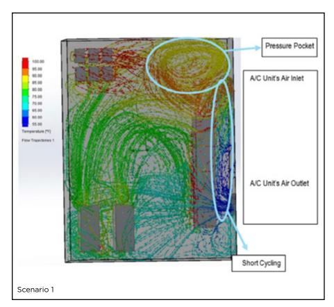
cooling. The two smaller drives in the corner are at risk of overheating, with the left one vulnerable as the right drive takes in cold air before it reaches the
