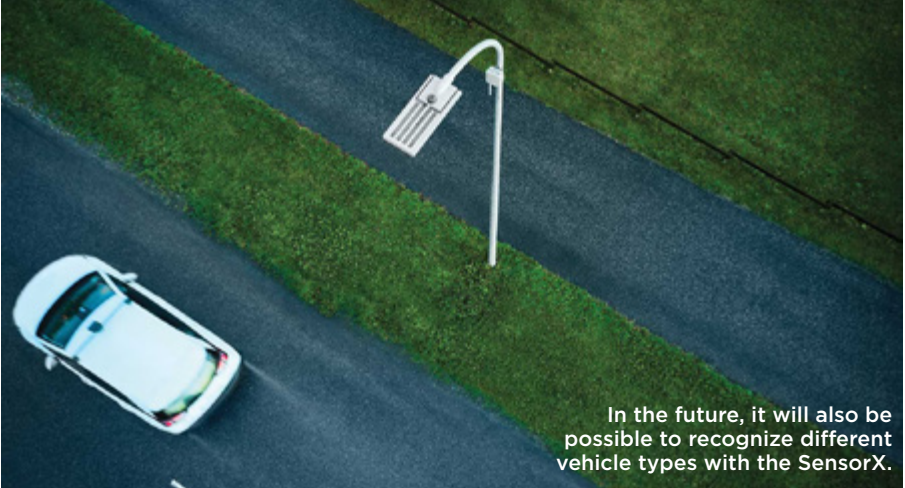
Tridonic's AI-based SensorX detects activity on roads and pavements so they can be accurately illuminated by street lights consuming minimal power.
