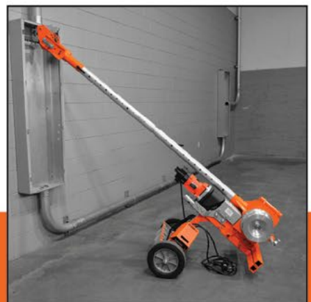
Overhead, underground and side pull capabilities.
