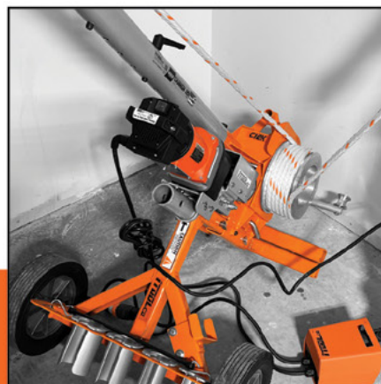
Dual capstans with a 3 speed motor.
