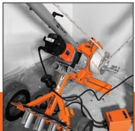
Dual capstans with a 3 speed motor.
